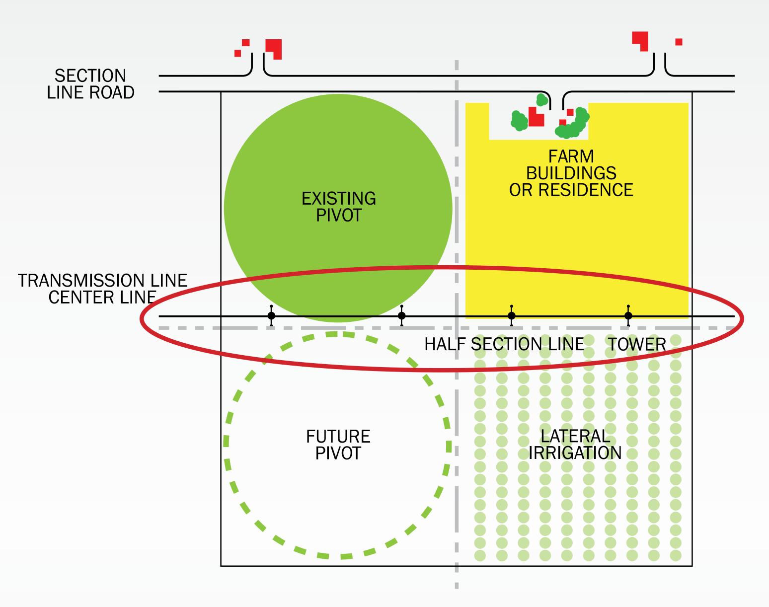
Location of line along half section maximizes avoidance of homes and farm buildings located along typical section line roads.
