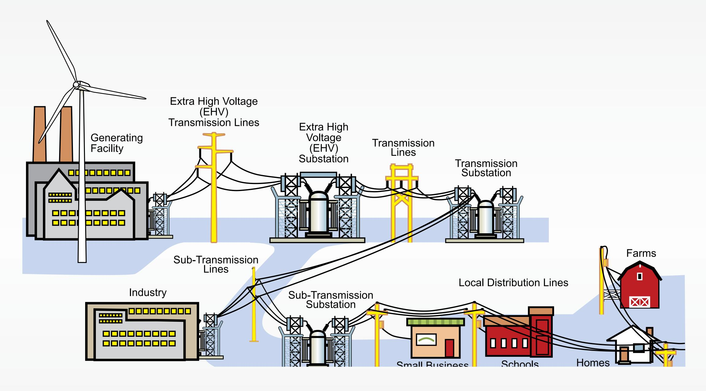
From the power plant, electric energy is delivered through a series of lines and substations where the voltage is reduced to the proper level for end-use customers.
